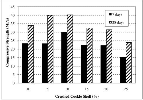
Fig.5: Effect of crushed cockle shell content on compressive strength of concrete at 28 days
