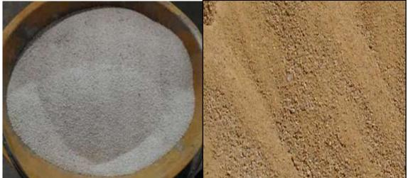
Fig.3: Crushed cockle shell to be used in concrete
